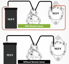
Remote Sense utilizes a second wire that reads the actual voltage at the battery. This signals the alternator to boost its output to compensate for the voltage drop, ensuring 14 Volts at the battery. The proper voltage forces more current into the battery bringing it to a full state of charge between vehicle stops.
