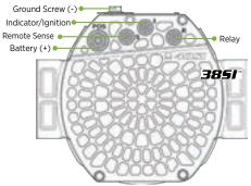
NOTE: When the Remote Sense terminal is not connected, the alternater operates and regulates voltage normally.
